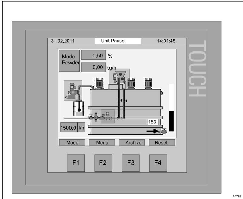
Fig. 18: System in operating mode [PAUSE]
