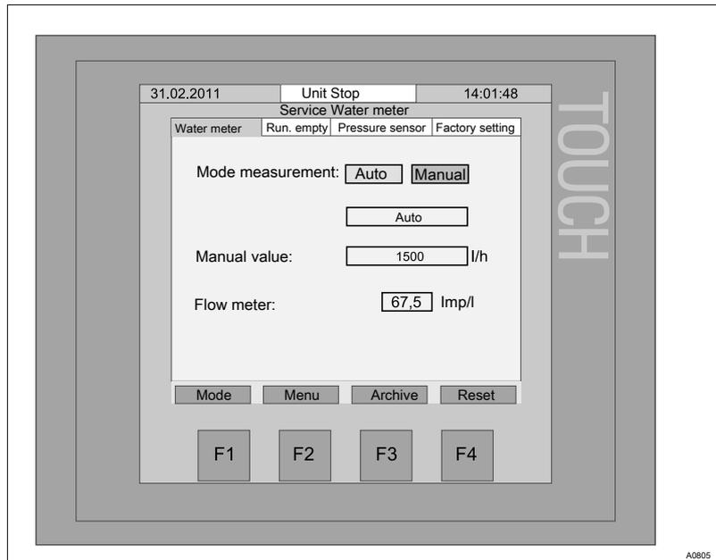
Fig. 39: Manual flow entry
