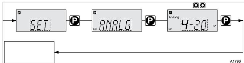
Fig. 11: [Analog] operating mode settings
