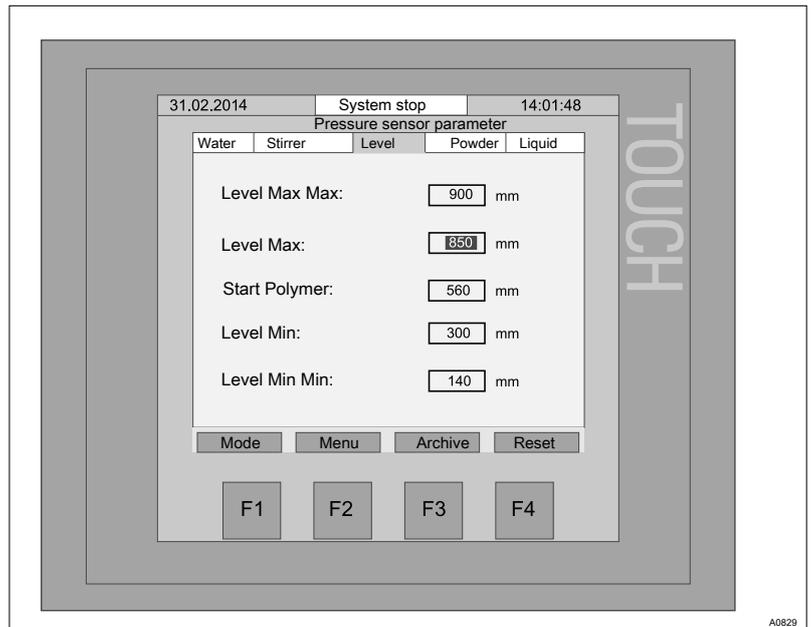
Fig. 27: Parameters [Level]
