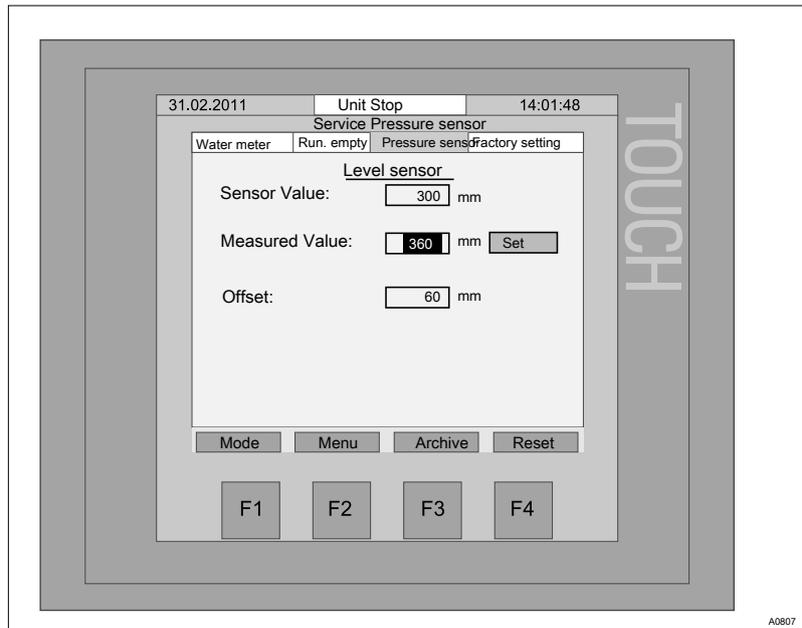
Fig. 41: Service - pressure sensor
