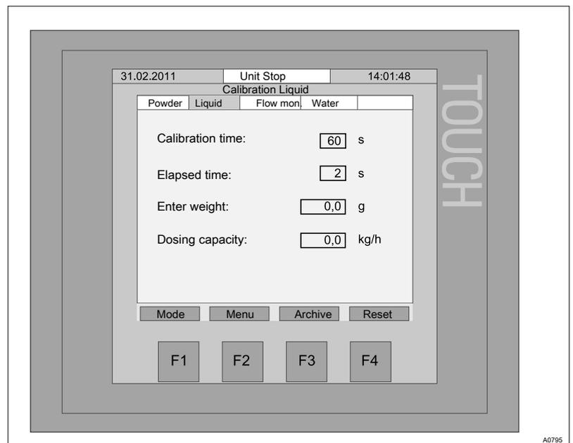
Fig. 29: Calibration liquid concentrate
