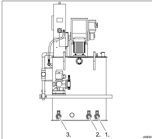
Fig. 5: Extraction openings
