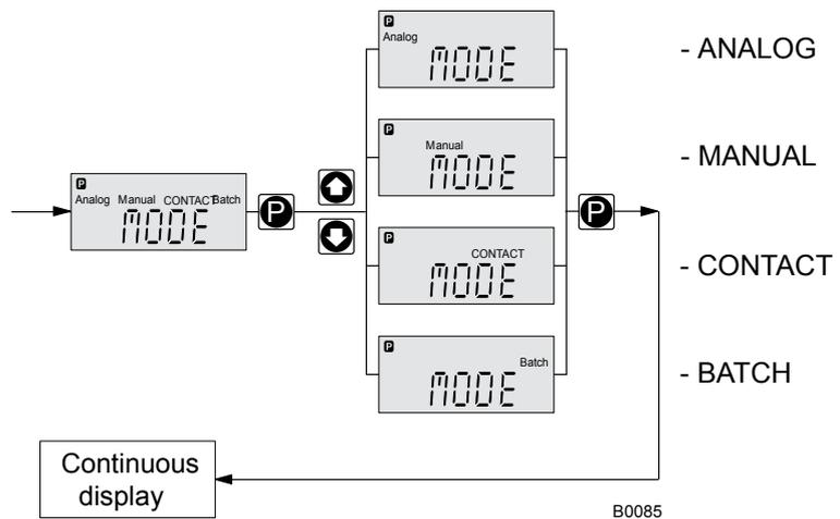
Fig. 10: Selecting the operating mode (MODE menu)
