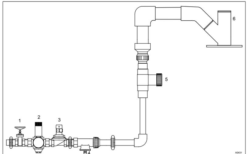
Fig. 6: Water fitting with Y-flush inlet
